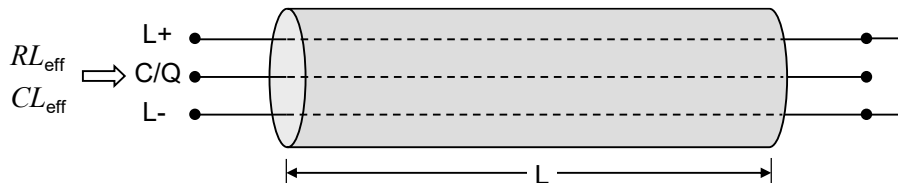
Figure 27 – Reference schematic for effective line capacitance and loop resistance
