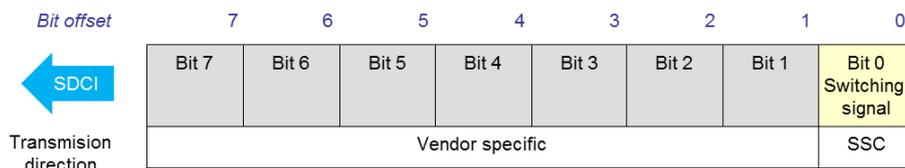
**Figure B.1 – 8 bit Process Data input structure with SSC**
