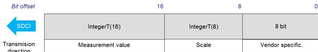
**Figure B.2 – 32 bit Process Data input structure**
